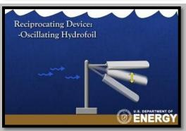
Reciprocating devices use the flow of water to produce lift or drag of an oscillating part of the device. This oscillation produces mechanical energy that feeds into a power conversion system.
